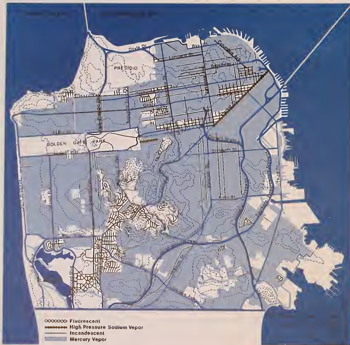
EXISTING STREET LIGHTING
